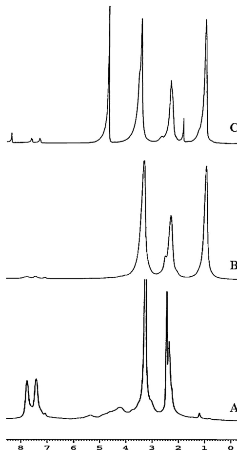
Fig. 3. ^1\text{H} NMR spectrum of (A) tosylated cellulose nanowhisker in DMSO- d_6 , (B) CNW-g-POX and (C) CNW-g-PEI.
